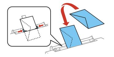
5. Push the paper or envelope down until it meets resistance. About 2 inches (5 cm) of the paper should be fed inside the printer as shown.
